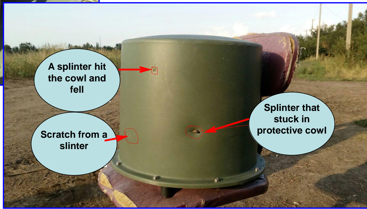
Damaged antenna cowl in a TCI 903S unit
